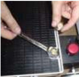
Replacing ship plug
